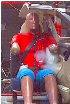
A modern car is equipped with a series of airbags (driver-, passengers-, side-impact-airbags), which are launched in a selective way in case of an accident. Out-of-Position situation (last picture). Courtesy of TRW.
