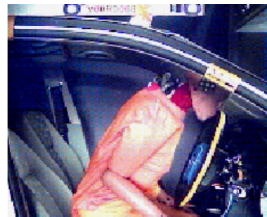
A modern car is equipped with a series of airbags (driver-, passengers-, side-impact-airbags), which are launched in a selective way in case of an accident. Out-of-Position situation (last picture). Courtesy of TRW.
